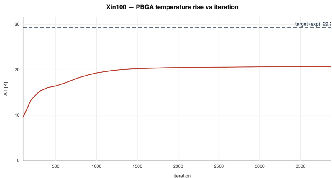
FIGURE 13. Package temperature-rise history \Delta T = T_{PBGA,avg} - T_{inlet} (Xin100).
